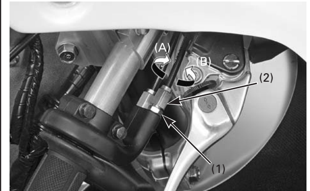
(1) LOCK NUT (2) ADJUSTER (A) DECREASE (B) INCREASE
